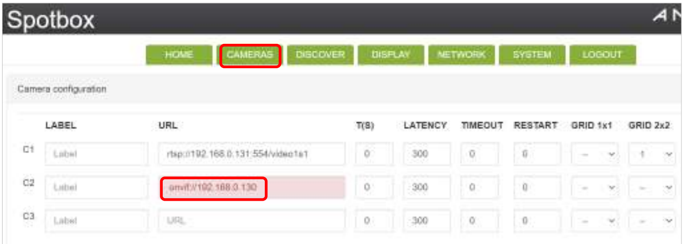
Figure 13 : CAMERAS tab - with incorrectly configure ONVIF camera
