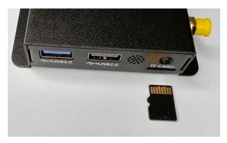
Once inserted correctly the micro SD card will lock in place, a further push on the SD card using you nail or other tool will unlock and eject it.
