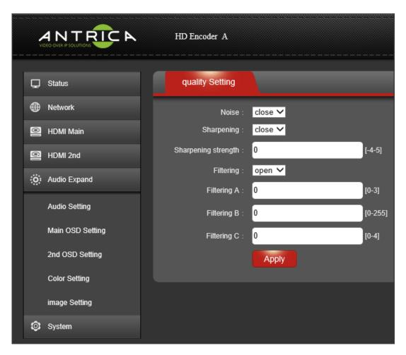
**NOISE**: Enable or disable a noise filter for removing white noise from camera images typically found on night time images.
