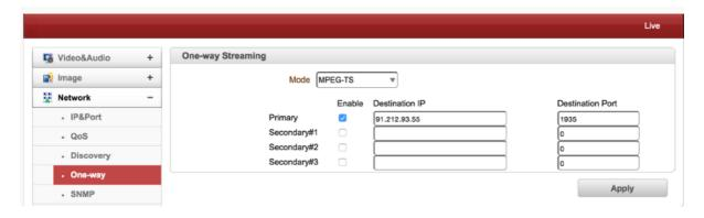
To stream MPEG TS first we need to setup ONE WAY STREAMING in the ANT-38500 which can be found under NETWORK-One way streaming.
