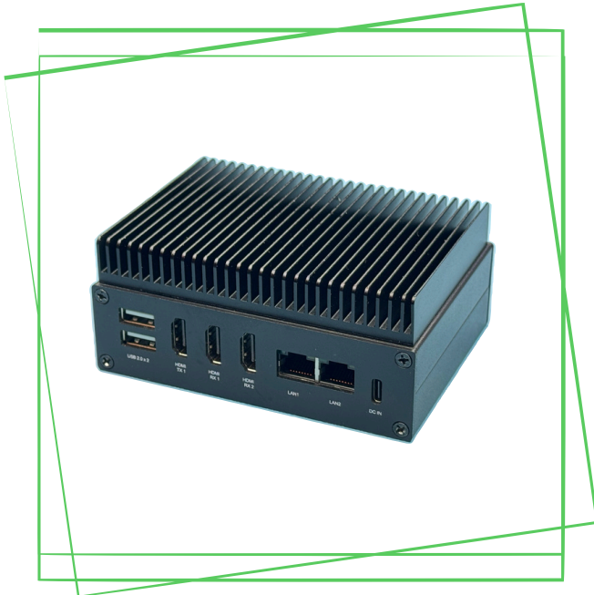
Ubuntu General purpose embedded computer with Docker Image environment; Upgradable with 4K H265/4 Video Encoder Customer hosted programs via Docker images
