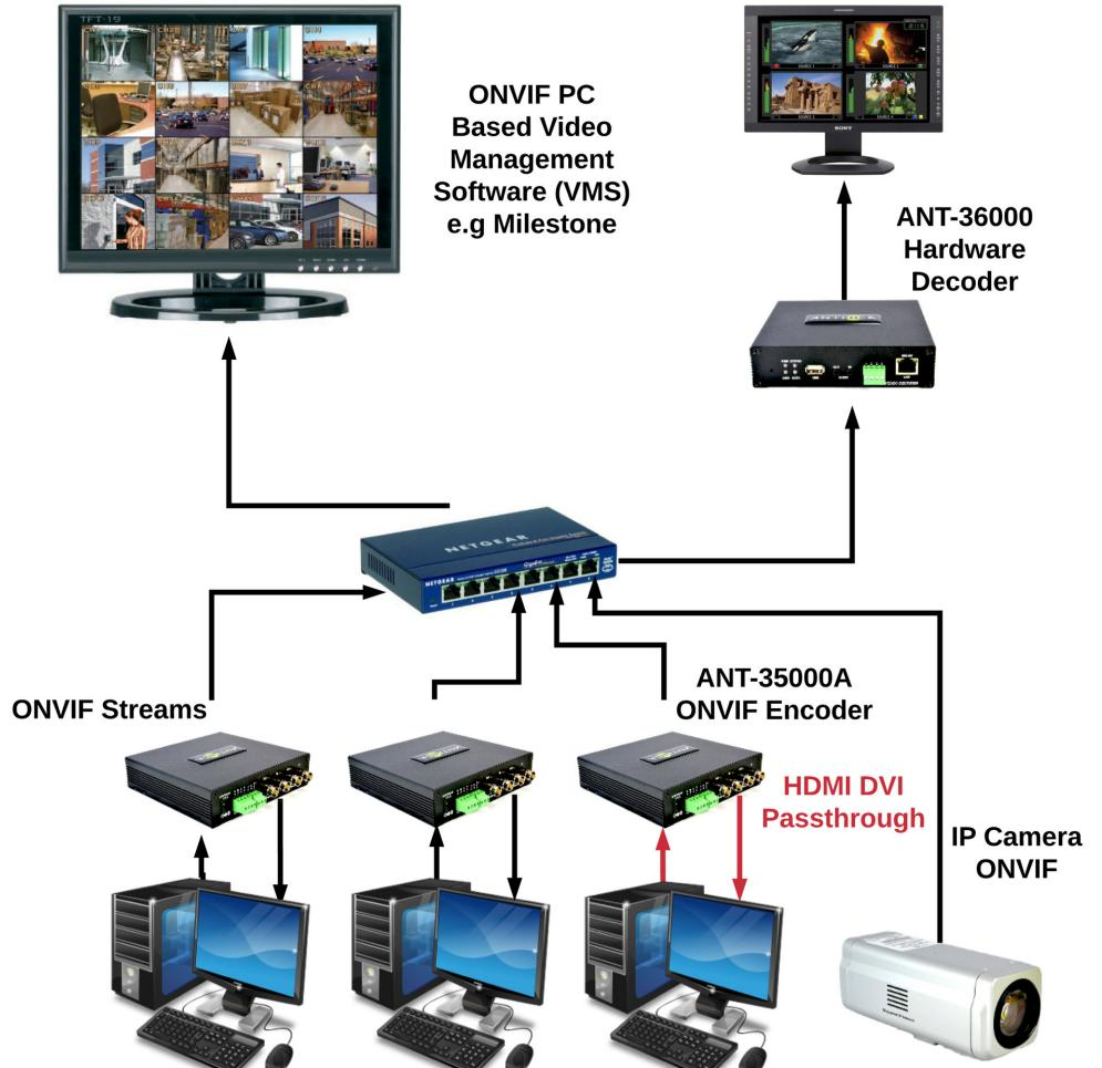
Description: Live religious events can be streamed over the internet to dedicated decoders located in remote communities (ANT-6000D). Video from cameras is encoded and streamed directly to individual places of worship. Alternatively streams can be uploaded directly to a YOUTUBE TV channel for wider audience viewing at home or on mobiles tablets etc.
