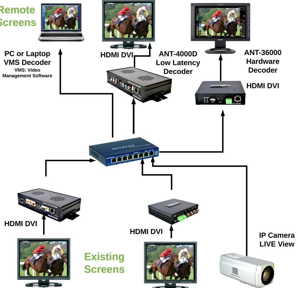
Description: Control Rooms use blade PC based decoders to decode multiple live streams and display them in various ways on a large video wall. By adding an ANT-35000A encoder any HDMI DVI HD-SDI signal can be encoded to an RTSP ONVIF stream for recording and viewing just like an IP camera. The ANT-35000A has a passthrough function so the PC output can be connected to the 35000A and then the passthrough connected to the LCD PC Monitor avoiding splitters.
