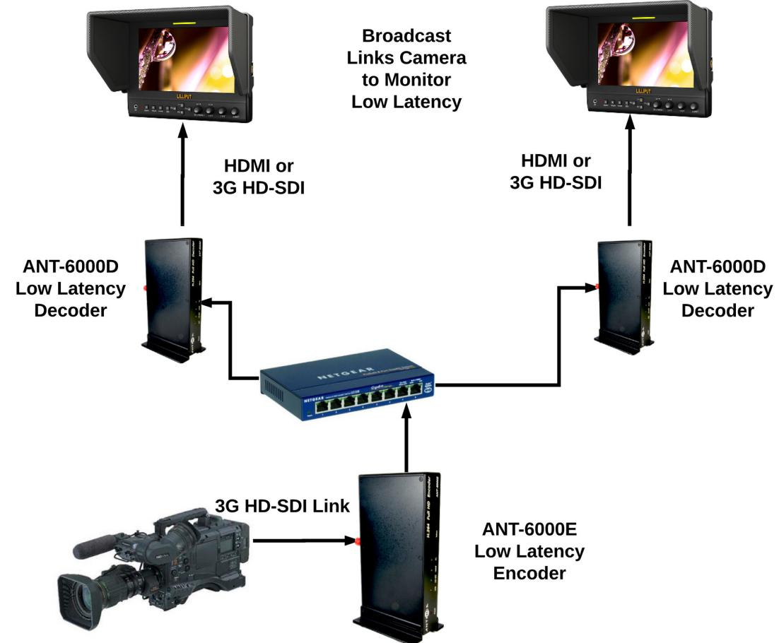
Description: Live events where the original view and sound can be seen and heard. In this situation any remote display needs to be connected via a low latency link. The ANT-6000 series provides a one to one or one to many connection over any 10/100/1000 LAN in around 100mS. Streaming to a dedicated decoder or broadcast to YouTube via RTMP streaming using the ANT-35000A encoder (not shown) or a dedicated IP camera with RTMP streaming as shown. HDMI or HD-SDI is supported up to 1080P60
