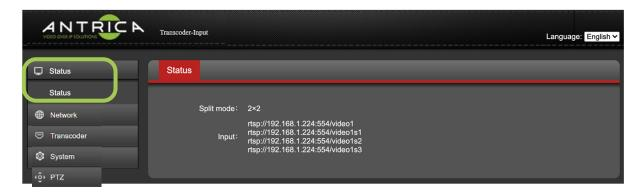
The status tab will show you information on the IP Input settings. This is effectively a decoder within the transcoder and can decode up to 4 streams or files. This screen will show if you are in 1x1 mode (1-1 transcode) or 2x2 mode (4 channels decoded and arranged as a quad image then transcoded). The input URLs or files are shown here
