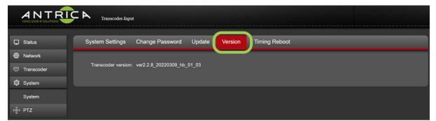
**Timing Reboot:** Allows the Decoder section to be rebooted automatically every N Hours ( 0-200 Hours)
