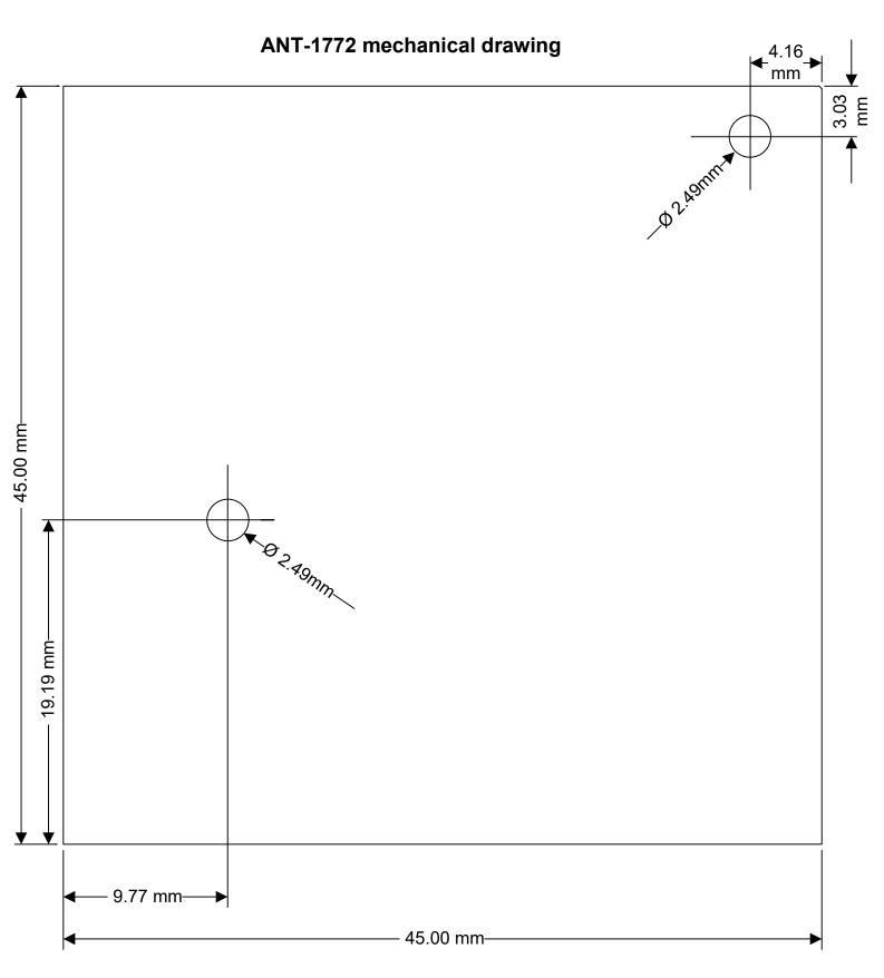
The required screw for the 2.49mm holes is a 2.5mm.
